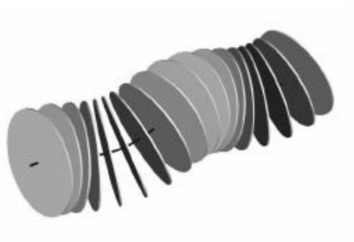
Figure 2: The perfect rope. Perpendicular sections of the rope are of the disk shape. None of the disks are allowed to overlap. This puts a limit not only on the spacial distance of different fragments of the curve into which the rope is shaped, but also on its local curvature.
