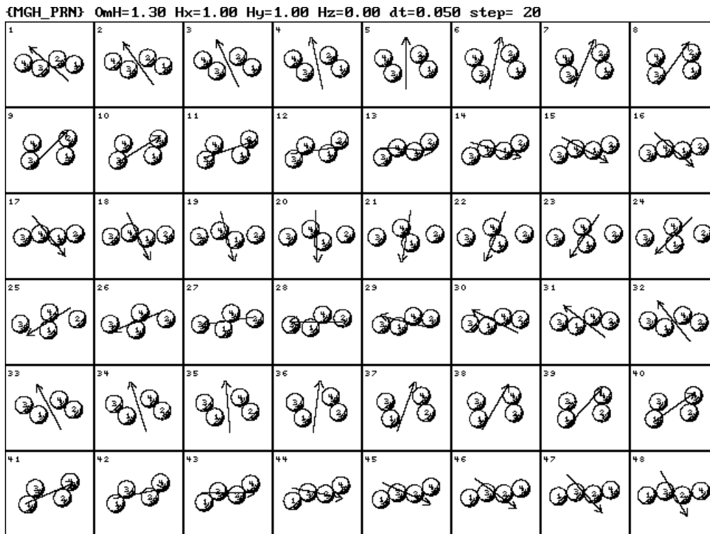
Fig.22 Sequence of frames taken from simulation of the M_2^{(4)} mode of motion as seen in the laboratory reference frame.
